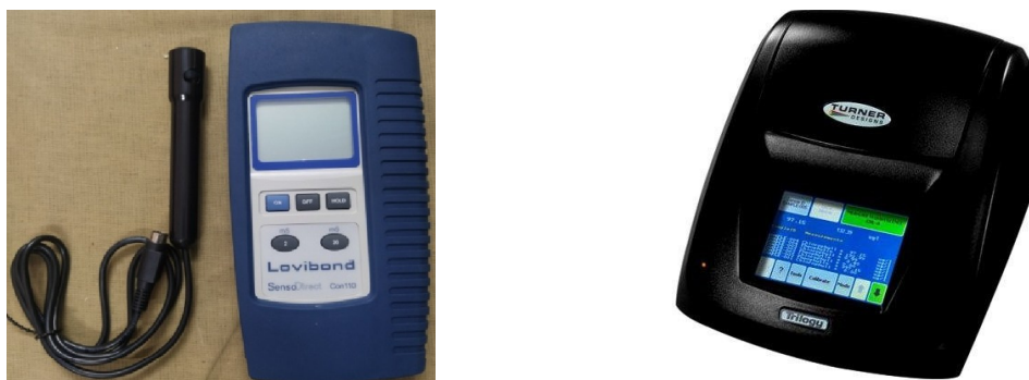
Fig. 2(a) Conductivity Meter with probe Fig.2(b): Image of Laboratory Fluorometer used for detection and analysis of dye tracer
